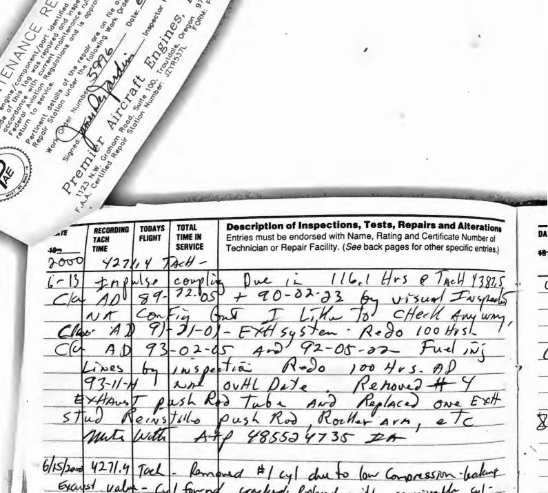
6/15/2000 4271.4 Tack - Removed # / cyl du to low Compression-leaking Excust value - Cyl formal cracked lopland with servicenth cylsee allow tool Premail Arcraft engines 40 5996. Instaled cylinhe with now cyl. box Oring, Now push rod seeds, New rocker cover gustot
