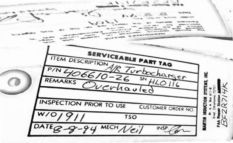
SERVICEABLE PART TAG ITEM DESCRIPTION D REMARKS Overhauled CUSTOMER ORDER NO. INSPECTION PRIOR TO USE TSO MECH
